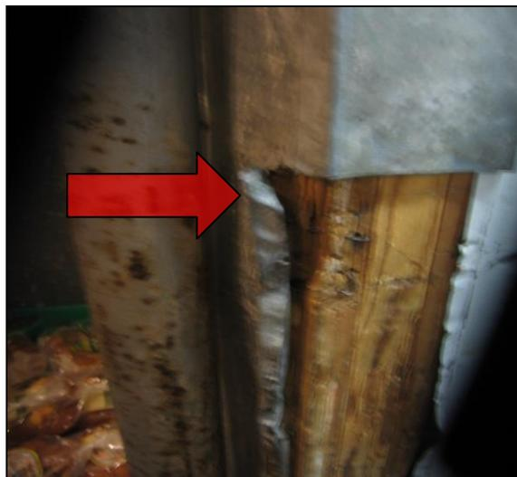
8. **Baler Lock Engagement Latch**- The baler door latch does not properly engage creating a hazard when lifting gate. When you lift the front gate the door should latch causing the door to stay open, however when the gate is raised the gate sometimes drops down which can create a pinch hazard for fingers and hands. Maintenance should fix baler door so door operates properly.
